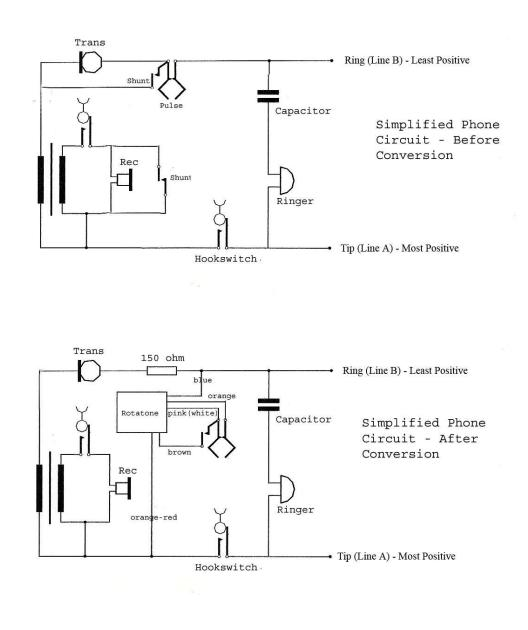
The above two diagrams above show a simple phone with a 'before and after' circuit. In order to operate Rotatone, the dial must have normally closed pulse contacts, and a contact that shorts to one of the pulse contacts when the dial is not at rest. There a relatively few dials that are not compatible with Rotatone.
